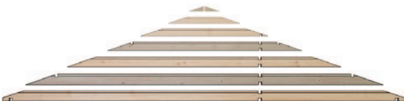
Gable board, C12 : 2 of 44 x 95 x 291mm Gable board, C11 : 1 of 44 x 145 x 1456mm Gable board, C10 : 1 of 44 x 145 x 2181mm Gable board, C9 : 1 of 44 x 145 x 3118mm Gable board, C8 : 1 of 44 x 145 x 3919mm Gable board, C7 : 1 of 44 x 145 x 4780mm Gable board, C6 : 1 of 44 x 145 x 5394mm
