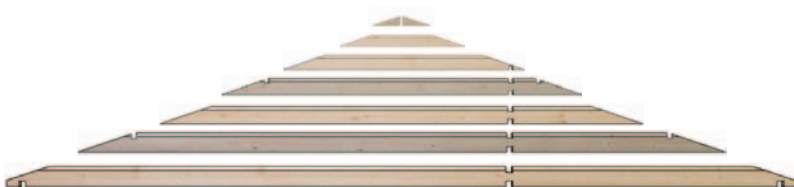
Gable board, E10 : 2 of 44 x 95 x 291mm Gable board, E9 : 1 of 44 x 145 x 1456mm Gable board, E8 : 1 of 44 x 145 x 2180mm Gable board, E7 : 1 of 44 x 145 x 3118mm Gable board, E6 : 1 of 44 x 145 x 3919mm Gable board, E5 : 1 of 44 x 145 x 4780mm Gable board, E4 : 1 of 44 x 145 x 5394mm
